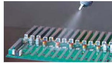
In-house conformal coating process
