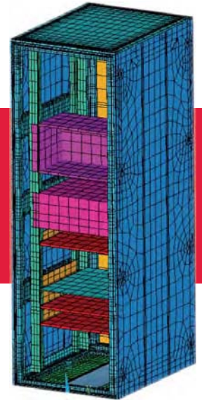
F.E. model - mesh and stress analysis
