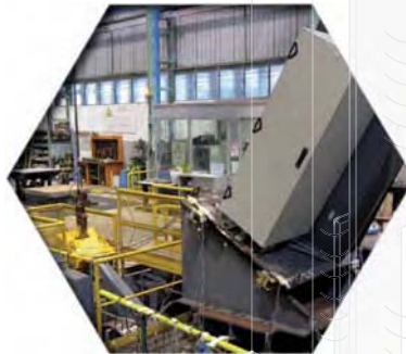
Cabinet tested to MIL-STD-901D
